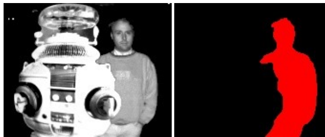
Fig 2. (Left) Intensity image from the SR-4000. (Right) Tracked and segmented human observer.
