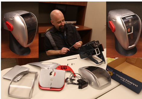
Figure 3: Usability test of SCIPRR by people representing the Expert HRI Mechanic persona. Subjects were given the head arrangement shown in the upper left and then directed to assemble into the new sensor configuration shown in the upper right.
