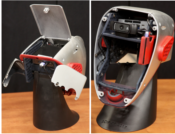
Figure 1: Design solution for a technology adaptable and social interaction affording robot head. The SCIPRR’s visor surface allows sensor penetration and facial expressions or data projection (Figure 2). The inner hex shaped scaffolding and easy access panels allows for easy configuration.
